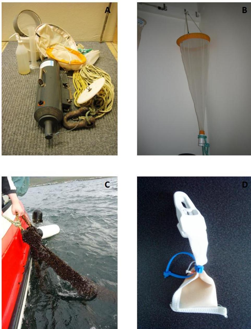
Figure 11: Sampling equipment (A) Niskin sampler, B) Plankton net, C) Mussel cages) and D) SPATT bag).
