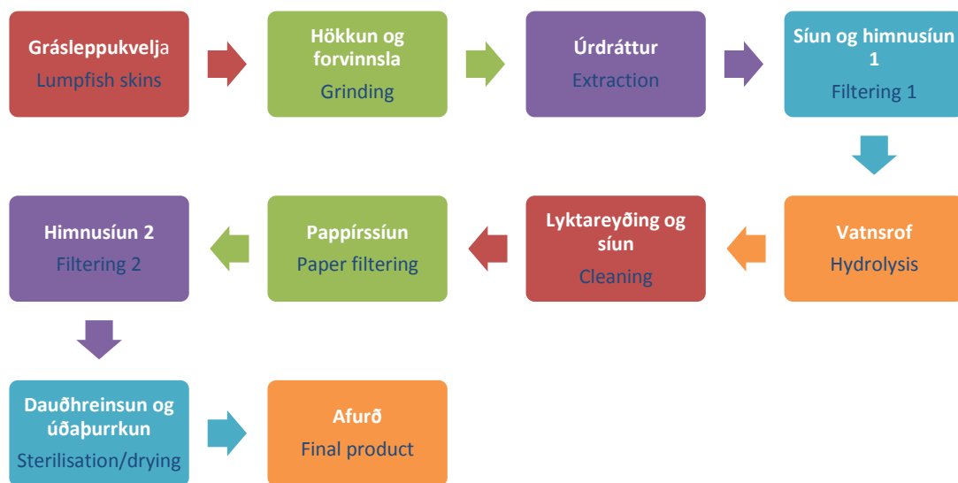
Mynd 5. Vinnsluferli kollagens hjá Seanergy í Færeyjum – The production process in the collagen factory in Faroe Islands.
